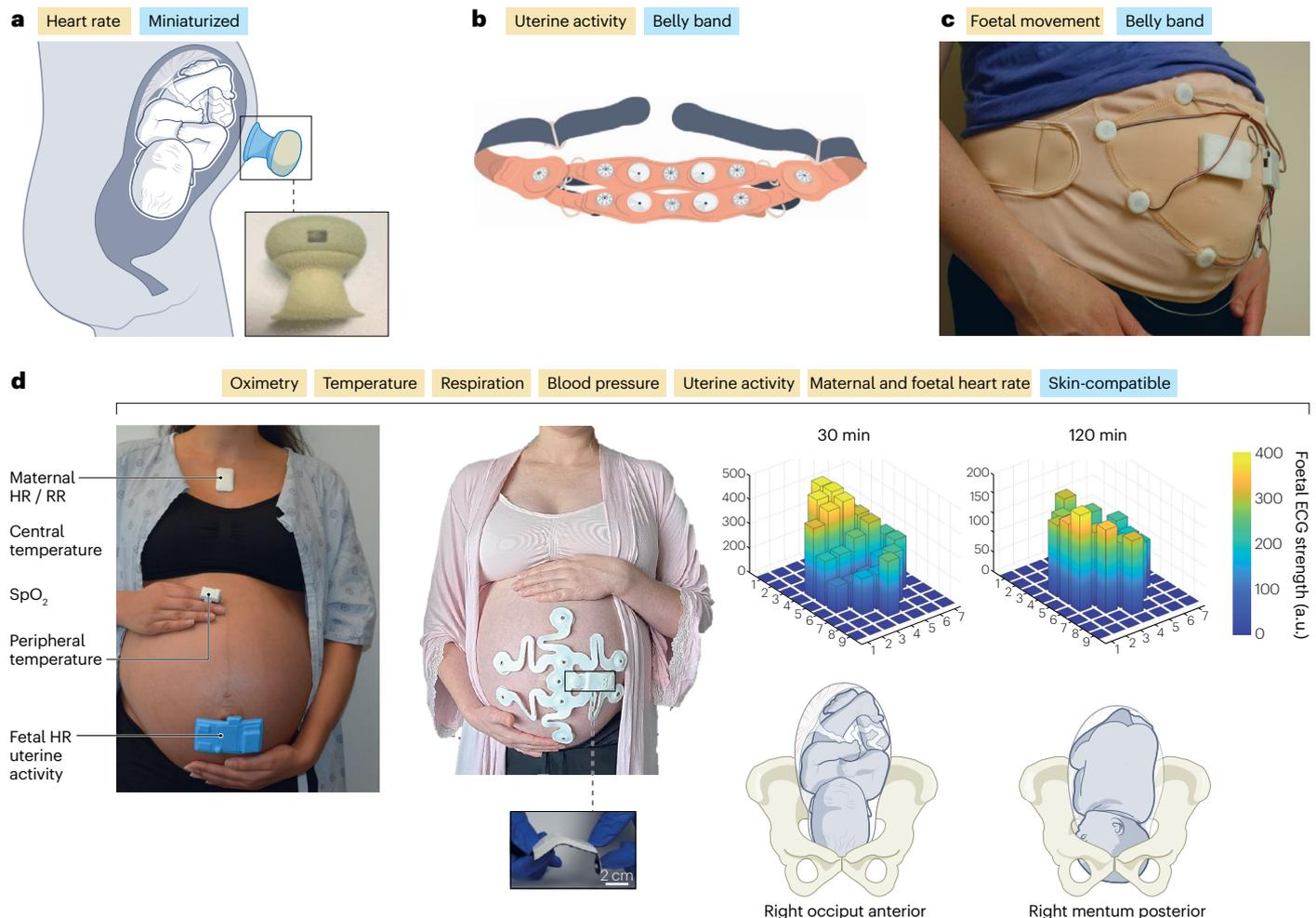
**Fig. 4 | Wireless biosensors for maternal and foetal monitoring.** **a**, A miniaturized portable wireless acoustic sensor system for monitoring FHR. **b**, A wearable pregnancy monitoring textile consisting of multiple ECG electrodes and acoustic sensors for monitoring FHR and uterine contractions. **c**, A wearable acoustic system with a tri-axial accelerometer for distinguishing foetal and maternal movements. **d**, An integrated wireless monitoring platform consisting of three
