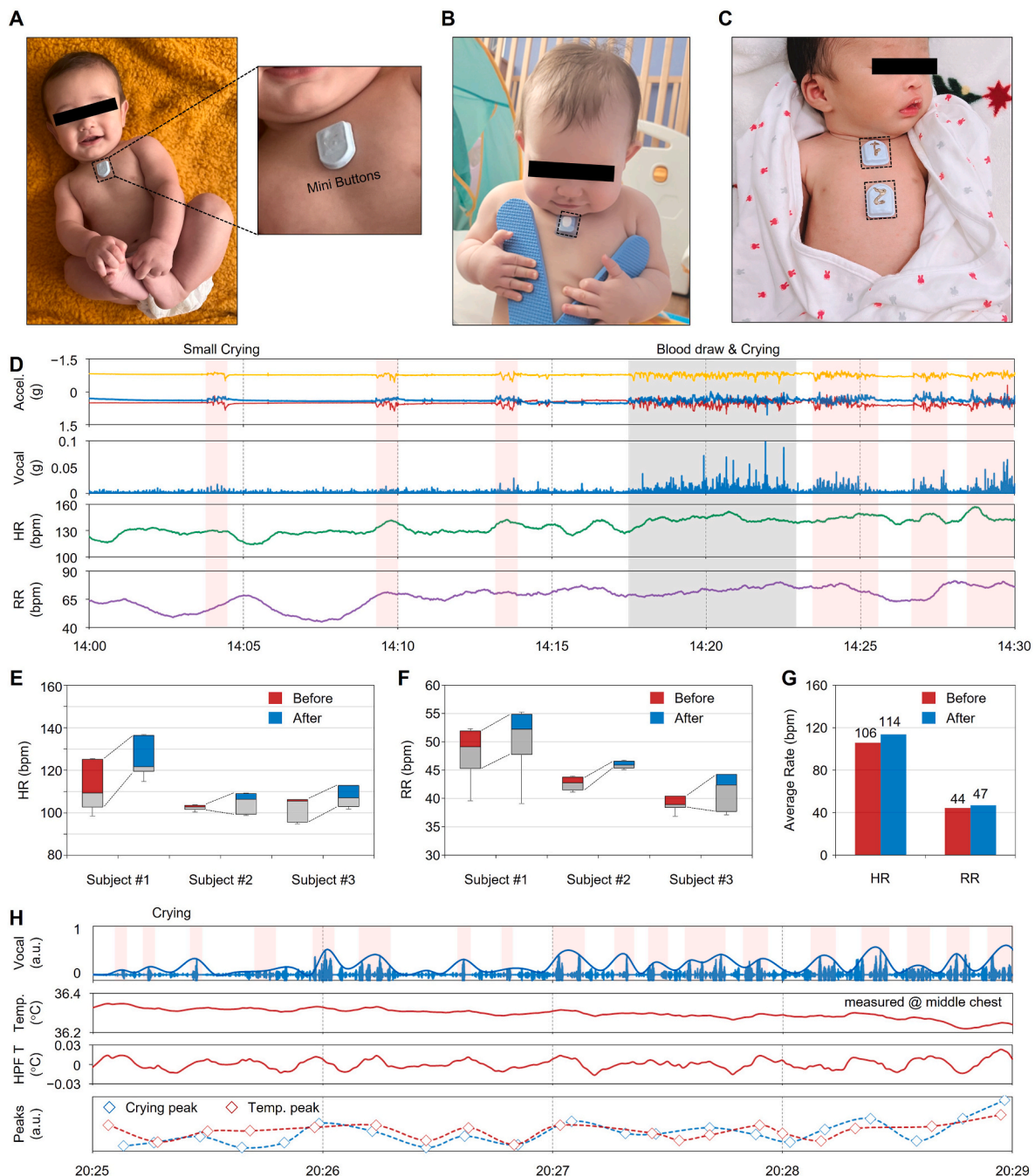
Fig. 6. (A)–(B) Photographs of infants mounted with a device on a suprasternal notch (SN) for tracking of cardiopulmonary activity. (C) Photograph of an infant mounted with two devices on alternative locations for collecting global movements of the body. (D) Representative data obtained from a neonate (gestational age, GA: 39 weeks) in the NICU before, during, and after a blood draw. (E)–(F) Corresponding HR and RR changes for three healthy infant subjects. (G) Average HR and RR data for 11 infant subjects. (H) Skin temperature data in response to crying for a newborn baby (GA: 42 weeks).
