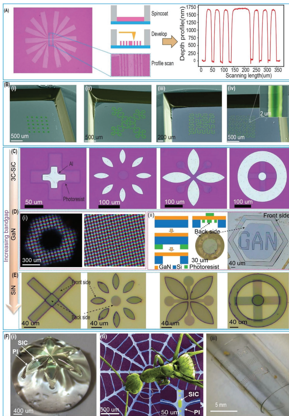
Figure 2. Micro-structures formed by back-side photolithography and double-side photolithography on free-standing SiC nanomembranes. A) Optical images of photoresist patterns on the back side of SiC free-standing membranes (right) and the corresponding step height profile (left), B) SEM images of different photoresist patterns on the back side of SiC free-standing membranes, C) Optical images showing good alignment of photoresist patterns on the back side and aluminium patterns on the front side of SiC free-standing membranes, D) Optical images showing: i) Excellent optical transparency of GaN membranes by observing smart phone pixels through a GaN membrane (left), and without GaN membranes (right), ii) the good alignment of photoresist patterns on the back side and aluminium patterns on the front side of GaN free-standing membranes, E) Optical images showing good alignment of photoresist patterns on the back side and aluminium patterns on the front side of SiN free-standing membranes F) Complex SiC structures on soft polymer substrates: i) Optical image of a SiC/ Polyimide (PI) flower on a water droplet ii) SEM images of a SiC/PI spider web structure with an ant on it iii) Optical image of serpentine SiC structures on a PDMS sheet bending on a tube.
