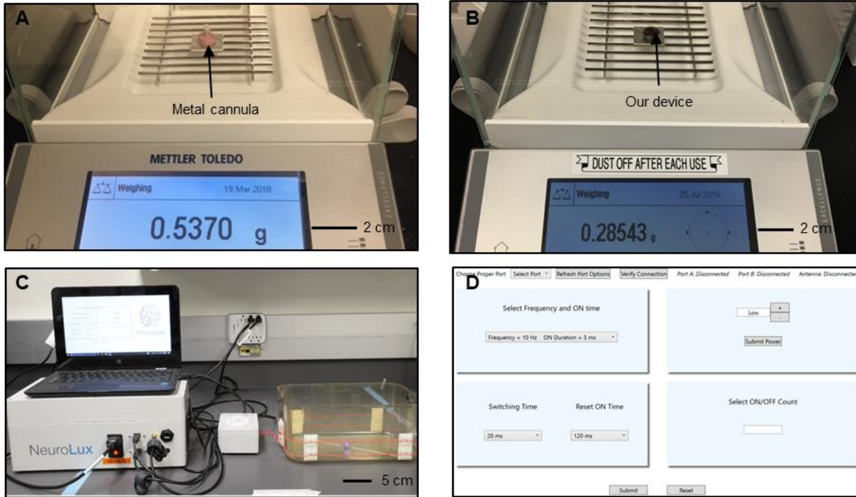
Fig. S1. Weight and complete hardware system of injectable optofluidic system. Weight of a conventional metal cannula (A) and a wireless, injectable optofluidic system (B). (C) Picture of the external hardware. (D) Screen image from a custom software application as a user interface.
