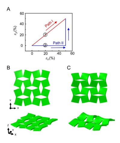
**Figure S14.** Wrinkle formation in elastomer substrates with square cut patterns during biaxial stretching. (A) Temporal sequence of changes in applied strains for two different loading paths. (B) Simultaneous biaxial stretching along path I in (A) does not create wrinkles while (C) sequential stretching along path II in (A) results in wrinkle formation. (B) and (C) correspond to the top-down and isometric views of state 1 and 2 shown in (A).
