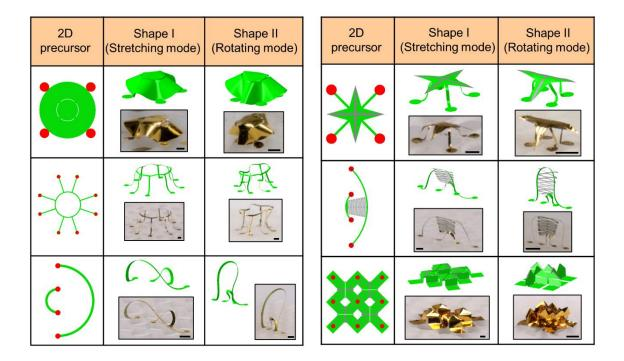
**Figure S5.** Incorporation of twisting into a broad set of 3D morphable mesostructures: 2D geometries, FEA predictions and experimental images (optical) of morphable 3D ribbon structures, membrane structures, and hybrid ribbon/membrane structures assembled on kirigami substrates. Shape I and shape II correspond to the 3D shapes after releasing of the stretching mode (prestrain from 100% to 40%) and releasing of the rotating mode (prestrain from 40% to 0%). Scale bars, 1 mm.
