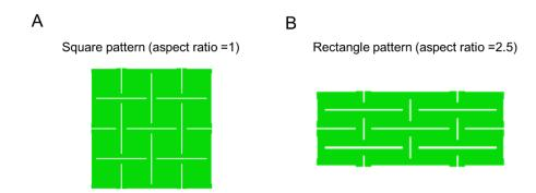
**Figure S13.** Schematic illustraions of (A) square cut pattern with a unit aspect ratio of 1 and (B) rectangular cut pattern with a unit aspect ratio of 2.5.
