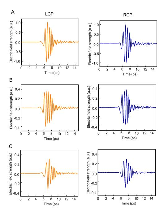
**Figure S16.** Measured THz electric field strength (arbitrary unit) as a function of time (unit: ps) under LCP and RCP for (*A*) blank, (*B*) shape I of the 3D trilayer microstructure (design I in Fig. 5*A*), and (*C*) shape II of the 3D trilayer microstructure.
