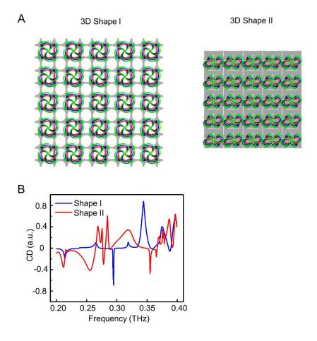
**Figure S17.** Simulations of an array of 3D morphable trilayer microstructures as mechanically tunable optical chiral metamaterials. (*A*) FEA results of a 5x5 array of 3D morphable trilayer microstructures (design I in Fig. 5*A*). (*B*) Electromagnetic simulation of the circular dichroism (*CD*) of an array of morphable 3D trilayer microstructures with two 3D shapes (design I in Fig. 5*A*) in the 0.2-0.4 THz frequency range.
