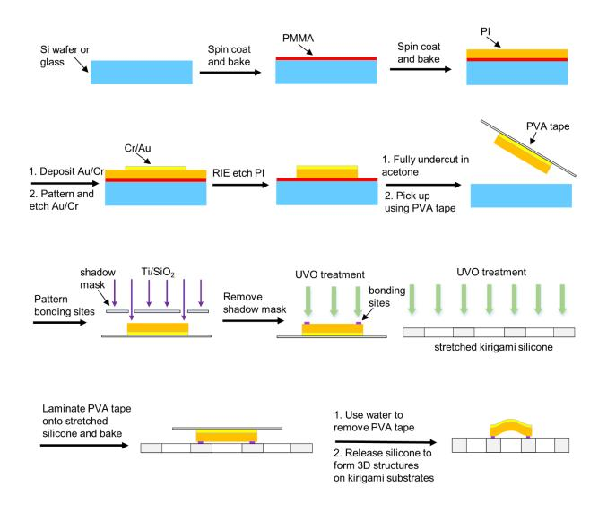
Figure S2. Schematic illustration of steps for fabricating 3D morphable structures on kirigami substrates.
