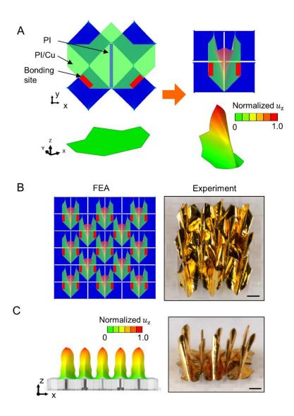
**Figure S9.** 2D geometries, FEA predictions and experimental images of an array of creased structures. (A) 2D precursor designs and FEA predictions (showing normalized displacements in z direction) of a unit creased structure before and after buckling and twisting. (B) Top-down view and (C) side view of FEA predictions and experimental images (optical) of an array of creased structures after buckling and twisting. Scale bars, 1 mm.
