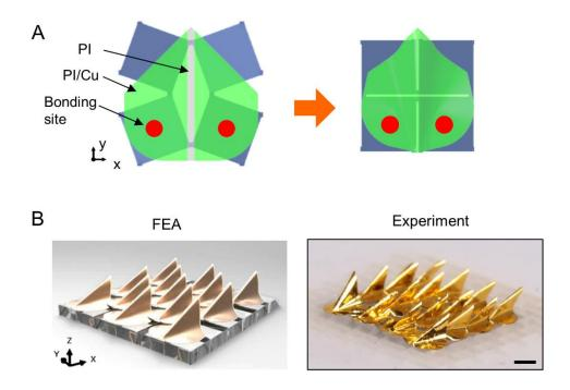
**Figure S10.** 2D geometries, FEA predictions and experimental images of a 4x4 array of creased structures. (*A*) Top-down view of 2D precursor designs and FEA predictions of a unit creased structure before and after buckling and twisting. (*B*) Isometric view of FEA predictions and experimental images (optical) of an array of creased structures after buckling and twisting. Scale bar, 1 mm.
