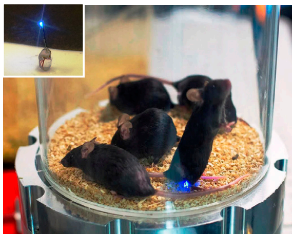
A resonant cavity (top) powers the wireless optogenetic platform developed by Ada Poon and colleagues at Stanford, using commercially available components. Wirelessly powered internal implants (inset, bottom) enable the mouse to move freely and behave normally while receiving optogenetic stimulation of peripheral nerve endings in the hind paw. A. Poon/Stanford University
