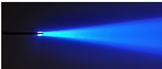
An optrode (an optical fiber glued to an electrode for measuring electrical activity of illuminated neurons) features a tapered electrode ending (left) for minimal tissue damage in larger brains of nonhuman primates during optogenetic stimulation. When switched on (right), the optrode emits a narrower, targeted cone of blue light.
