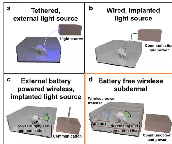
FIG. 1. Schematic illustrations of options in neuroscience tools designed for freely moving subjects. (a) Tethered, fiber optic interface to an external light source for optical stimulus and recording. (b) Tethered, wired interface to an implanted light source, with options in multichannel recording and stimulation. (c) External, battery-powered wireless system with an implanted light source. (d) Battery-free subdermal implant.
