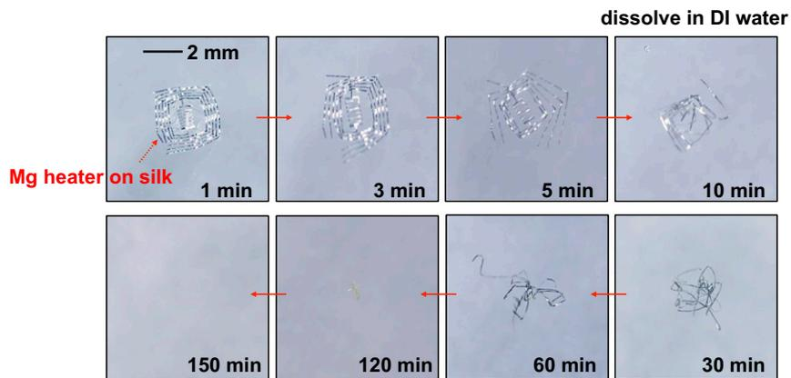
Fig. S3. Optical images of full dissolution of the bare device (i.e., without any encapsulation layer) in DI water at room temperature over a time interval of 2.5 hours.
