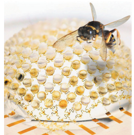
Figure 1 | Insect-inspired visual sensor. Song et al. 1 have designed a visual sensor that resembles, both functionally and structurally, the apposition eye of a daylight insect.
