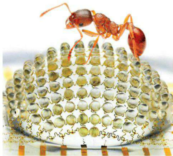
Rogers and colleagues' compound camera lens is modeled after the eye of an ant (shown to scale in this composite illustration), giving it a wide field of view and acute motion-sensing capability.
