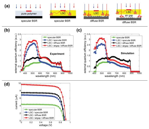
**Figure 3.** a) Schematic illustrations of GaAs  $\mu$ -cells embedded on the surfaces of different LSCs. b) Measured EQE spectra. c) Simulated EQE spectra. d) Measured current-voltage (I–V) characteristics under AM1.5G illumination. Substrates: PU/ specular BSR (green triangle), LSC/ specular BSR (blue square), LSC/ diffuse BSR (black diamond), LSC/ air gap/ diffuse BSR (red circle).
