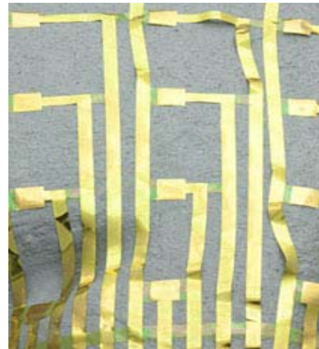
Neural electrode array wrapped onto a model of the brain. The wrapping process occurs spontaneously, driven by dissolution of a thin, supporting substrate of silk.
