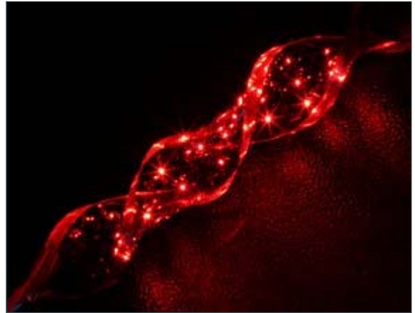
The LEDs can be twisted into a 720-degree helix (Source: University of Illinois)
