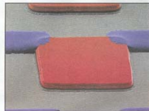
Microscope image of an ultrathin, micro-LED (red) in a suspended, 'diving board' layout, released along its bottom surface from the growth wafer (grey), but held in place with polymer 'anchor' structures (blue) at the two back corners.
