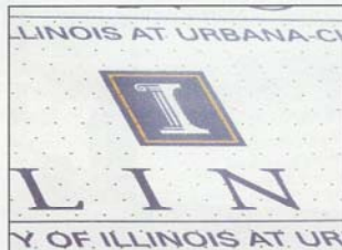
Array of ultrathin, micro-LEDs (black squares) printed onto a plate of glass, with a university logo pattern in the background.
