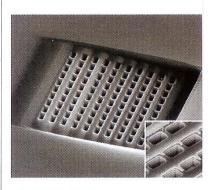
LIGHT BENDING An image produced by a scanning electron microscope shows a wedge-shaped prism. The device was carved from layers of metal and insulating material (inset) punched with rectilinear holes.
