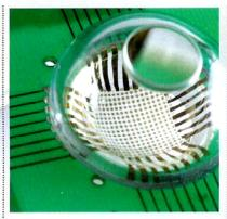
semiconductor wafers or glass plates and, in more recent work, flat plastic sheets and slabs of rubber. None are suitable for the eye-camera application contemplated here because of the mechanical strains needed to accomplish the hemispherical geometry are too large. They just would not be able to bend into shape without fracturing the circuit materials," Rogers says. "Fully stretchable electronics, on the other hand."
