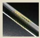
← ELASTIC substratemounted silicon circuits can conform to objects with a relatively small radii of curvature—in this case, 2mm.
