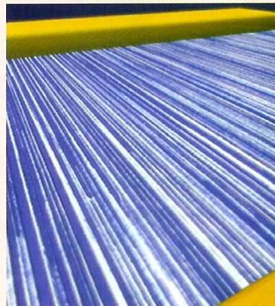
Colorized scanning electron micrograph of an SWNT array (blue and white) with artist drawings of the device electrodes (gold). (Courtesy of John A. Rogers.)
