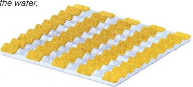
Releasing the tension on the elastic produces “waves” of silicon that can later be stretched out again as needed. Such flexible silicon could be used to make wearable electronics.
