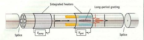
Integrated heaters manipulate the position (pump) and temperature (grating) of two plugs of liquid within microchannels around the fiber core. The position of the high/low refractiveindex boundary determines the depth of the notch filter (increasing from left to right). Changing the temperature across the grating from 25°C to 16°C changes filtered wavelength from 1545 to 1555 nm.
