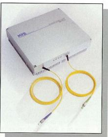
The Super Raman Fiber Laser from Montreal-based MPB Communications Inc. is a pump source that provides distributed Raman amplification in transmission spans of telecommunications systems via third-order cascaded Raman pumping. Third-order cascaded Raman amplification of C-band signals requires launching high power at 1276 nm, the third-order pump wavelength, and low seed powers at about 1356 and 1455 nm, the intermediate and final pump wavelengths.
