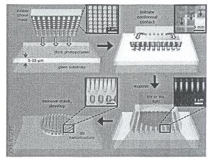
Clockwise from the upper left: A rubber phase mask is placed on a photopolymer, where it sticks due to atomic forces. The system is exposed, the mask removed, and the photoresist developed, leaving a 3-D structure.
