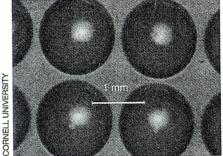
Replicated lenses with a pitch of 1.25 mm are arrayed on a quartz backing plate (top and bottom); the central 10 × 10 section of the  $12 \times 12$  array is usable.
