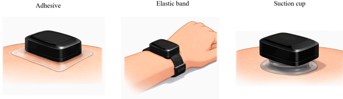
Fig. 1. Schematic illustration of different mounting methods, including adhesive interfaces and adhesive-free interfaces (with elastic band or suction cup).
