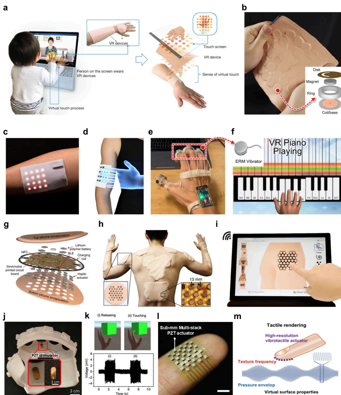
Figure 9. Vibrotactile feedback devices. (a) Skin-integrated vibrotactile haptic device for social communication scenario. (b) Vibrotactile haptic actuators based on LRAs utilizing Lorenz forces. Inset: exploded view of the vibrotactile actuator. Reproduced with permission from ref 31. Copyright 2019 Springer Nature. (c) Haptic feedback patch with self-sensing mechanism employing Faraday's law. (d) Reproduction of virtual touch via LRA-based haptic feedback patch. Reproduced with permission from ref 156. Copyright 2022 The American Association for the Advancement of Science under CC BY 4.0 license https://creativecommons.org/licenses/by/4.0/ . (e) Wearable tactile feedback device using ERM vibrators. (f) Demonstration of a piano training application in a VR environment. Inset: Optical image of the ERM vibrator. Reproduced with permission from ref 253. Copyright 2022 Springer Nature under CC BY 4.0 license https://creativecommons.org/licenses/by/4.0/ . (g) Schematic of a haptic interface composed of ERM motor array. (h) Digital image of the haptic interface delivering vibrotactile sensations to large areas of various body parts. (i) Wireless touch transmission through spatiotemporal vibration stimulation by individually controlling ERM motors. Reproduced with permission from ref 254. Copyright 2022 Springer Nature. (j) Smart glove providing precise vibrational feedback via piezoelectric.
