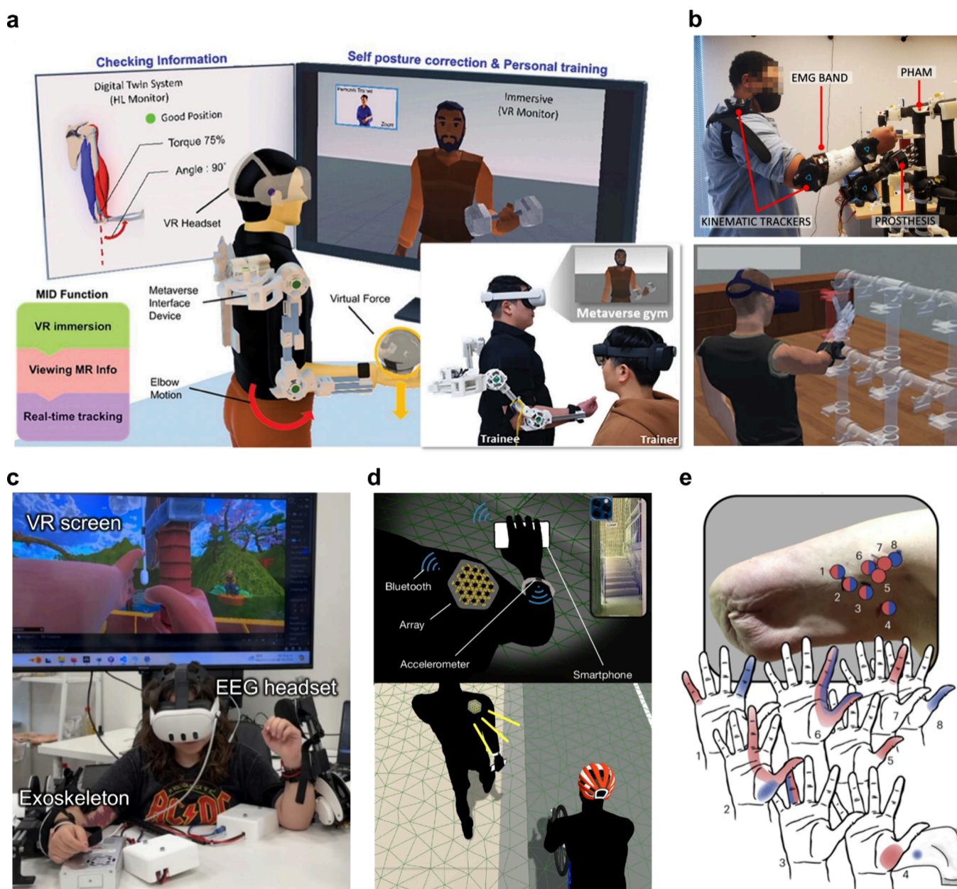
Figure 36. Application of wearable XR devices for rehabilitation and sensory substitution. (a) Hybrid upper-arm exoskeleton system integrated with an anatomical digital twin, enabling immersive rehabilitation. Inset: the scenario enables the trainer and trainee to interact using extended reality. Reproduced with permission from ref 834. Copyright 2023 Wiley-VCH. (b) MR-based rehabilitation system assisting patients in training arm strength and balance control. Optical image of patient undergoing rehabilitation with equipment in the real world (top) and corresponding VR image (bottom). Reproduced with permission from ref 813. Copyright 2023 Springer Nature under CC BY 4.0 license https://creativecommons.org/licenses/by/4.0/ . (c) Real-time integration of EEG headset, upper-limb exoskeleton, and VR interface for cognitive-motor rehabilitation using motor imagery-based control. Reproduced with permission from ref 835. Copyright 2025 MDPI under CC BY 4.0 license https://creativecommons.org/licenses/by/4.0/ . (d) Skin-integrated haptic system designed for sensory substitution, delivering structured feedback to assist perception and motor control in users with sensory impairments. Reproduced with permission from ref 199. Copyright 2024 Springer Nature. (e) Wearable thermal feedback TED for neurological rehabilitation. Reproduced with permission from ref 335. Copyright 2023 Springer Nature.
