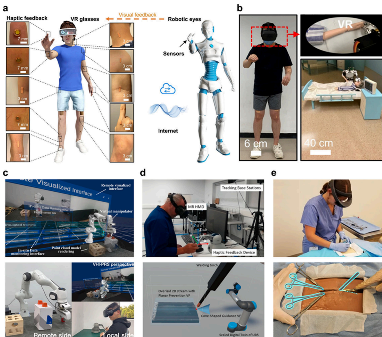
Figure 34. Application of wearable XR devices for work assistance. (a) Soft wearable XR devices integrated with haptic actuators and high-resolution VR glasses to provide multiple forms of feedback. A user remotely controlling a robot through glasses and feedback devices (left). A robot being remotely controlled by the user (right). (b) Application of teleoperation technology that enables remote interaction with equipment located in distant or physically inaccessible areas. User controlling remotely (left), view through VR glasses (top right), and remote patient care using a robot (bottom right) (scale bars: 6 cm, 40 cm). Reproduced with permission from ref 206. Copyright 2022 The American Association for the Advancement of Science. (c) Robotic arm system for remotely controlling industrial manipulators through visual and haptic feedback devices. Images of the system in the VR environment (top), robotic arm on the remote side (bottom left), and user operating the system (bottom right). Reproduced with permission from ref 805. Copyright 2024 Elsevier. (d) Intuitive remote welding robot with MR devices (top) and welding operation in MR interface (bottom). Reproduced with permission from ref 804. Copyright 2021 Multidisciplinary Digital Publishing Institute under CC BY 4.0 license https://creativecommons.org/licenses/by/4.0/ . (e) AR Surgical telementoring. Medical professionals wearing VR headsets (top) and first-person view of medical professionals wearing VR headsets and 3D surgical guidance from remote experts (bottom). Reproduced with permission from ref 803. Copyright 2020 Springer Nature under CC BY 4.0 license https://creativecommons.org/licenses/by/4.0/ .
