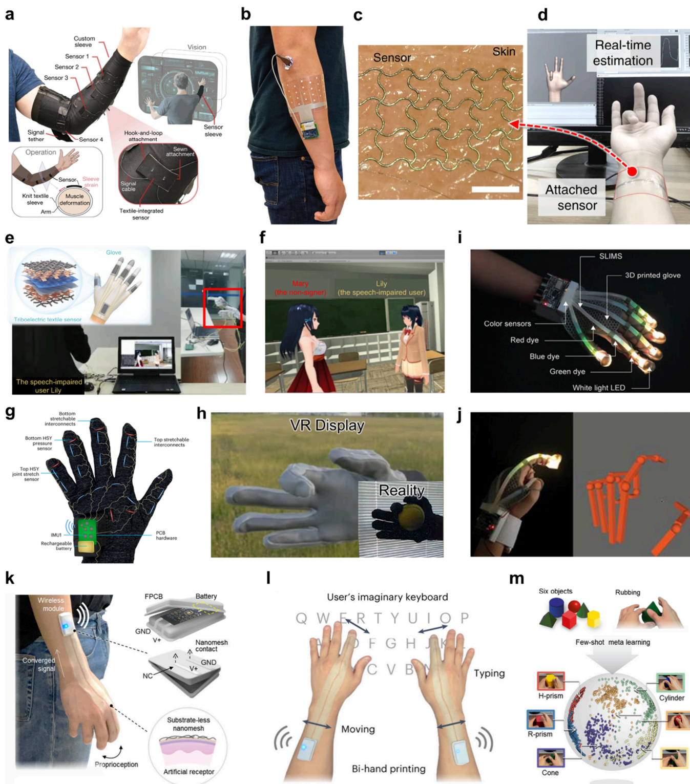
Figure 23. Gesture recognition systems. (a) Strain-based gesture recognition system that measures muscle deformation to classify various hand gestures. Inset: schematic illustration of the system in operation (left) and magnified image showing a strain sensor of the system (right). Reproduced with permission from ref 544. Copyright 2020 Springer Nature. (b) EMG-based gesture recognition system worn on the forearm with 64-channel soft electrodes. Reproduced with permission from ref 197. Copyright 2020 Springer Nature. (c) Skin-integrated strain sensor based on controlled crack structure (scale bar: 1 mm). (d) Estimation of finger movements based on subtle deformations of wrist skin. Reproduced with permission from ref 542. Copyright 2020 Springer Nature under CC BY 4.0 license https://creativecommons.org/licenses/by/4.0/ . (e) Communication scenario where sign language in the real world is converted into text and audio in a VR environment through triboelectric textile sensors. Inset: exploded view of textile sensors detecting strain and touch on the fingers for gesture recognition. (f) VR interaction between a speech-impaired user and a nondisabled user, enabled by real-time sign language recognition and audiovisual translation. Reproduced with permission from ref 553. Copyright 2021 Springer Nature under CC BY 4.0 license https://creativecommons.org/licenses/by/4.0/ . (g) Smart gloves integrated with yarn-based sensors measuring the bending angle and grasping pressure of the fingers. (h) Finger movements in the VR
