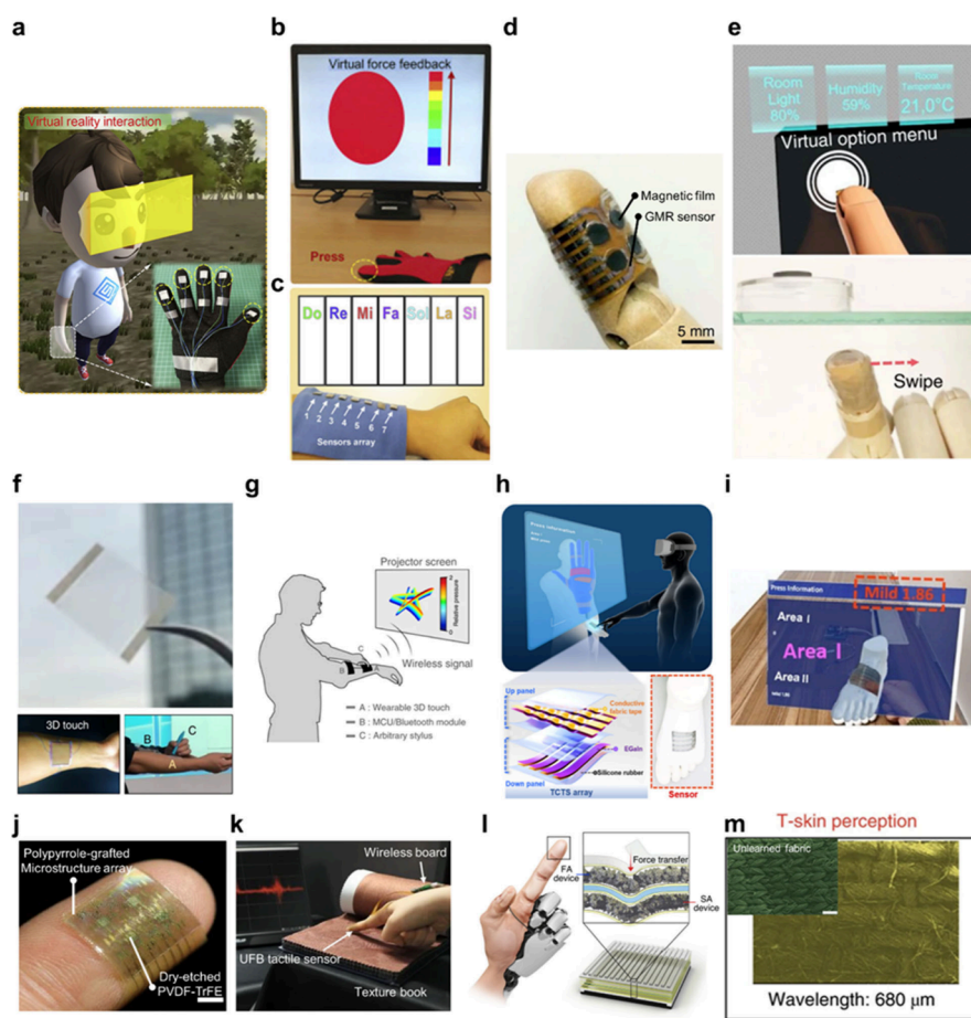
Figure 22. Touch sensing devices. (a) Interactive virtual application through a haptic interface integrated with tactile sensors. Inset: the haptic interface worn on the hand. (b) Virtual force feedback represented by color changes according to the detected pressing force. (c) Demonstration of virtual piano that provides sound with varying pitch and levels based on the sensing signals. Reproduced with permission from ref 464. Copyright 2019 Elsevier. (d) Tactile sensors composed of a magnetic film with a bump structure and a GMR film (scale bar: 5 mm). (e) Graphic (top) and optical (bottom) images of an AR scenario where the user explores and selects a virtual option menu. Reproduced with permission from ref 465. Copyright 2019 Springer Nature under CC BY 4.0 license https://creativecommons.org/licenses/by/4.0/ . (f) Transparent touch sensor for collecting 3D information (top). Images of the touch sensor attached to the arm (bottom left) and the device being used to draw (bottom right). (g) Schematic illustration showing wireless transmission of shapes drawn on the skin. Reproduced with permission from ref 466. Copyright 2019 Springer Nature under CC BY 4.0 license https://creativecommons.org/licenses/by/4.0/ . (h) Bimodal touch sensor that recognizes both static and dynamic tactile signals. (i) Schematic of MR application displaying the pressed area and the pressure intensity. Reproduced with permission from ref 467. Copyright 2024 American Chemical Society under CC BY 4.0 license https://creativecommons.org/licenses/by/4.0/ . (j) Tactile sensory system based on resistive and piezoelectric sensors for acquiring static and dynamic pressure information, respectively (scale bar: 2 mm). (k) Digital image of the tactile sensory system collecting texture information from various fabrics. Reproduced with permission from ref 222. Copyright 2022 Springer Nature. (l) Touch sensing device mimicking SA and RA mechanoreceptors. Inset: schematic showing the force sensing mechanism of the device. (m) Classification result of unlearned fabric using texture information obtained through the sensing device. Inset: the image of the unlearned fabric. Reproduced with permission from ref 447. Copyright 2021 Springer Nature.
