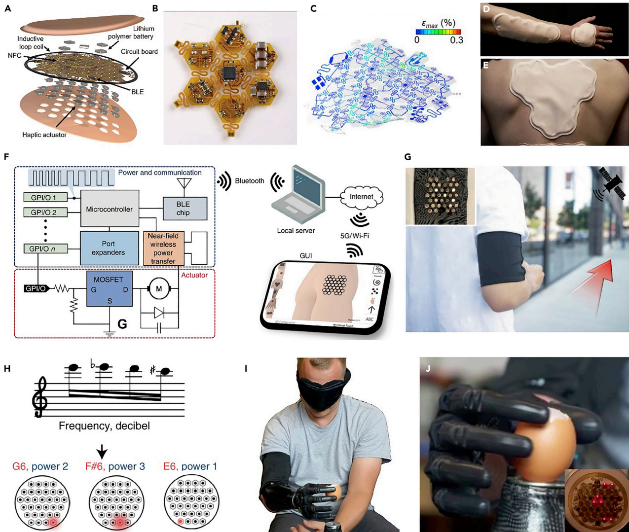
Figure 1. Design and applications of the wireless haptic interface
