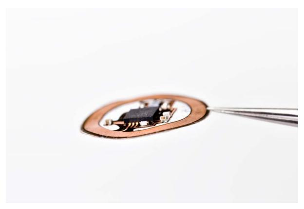
Sweat enters the device through tiny holes and flows through a network of microchannels, each the width of a hair. Sensors detect specific chemicals such as glucose and lactate.
