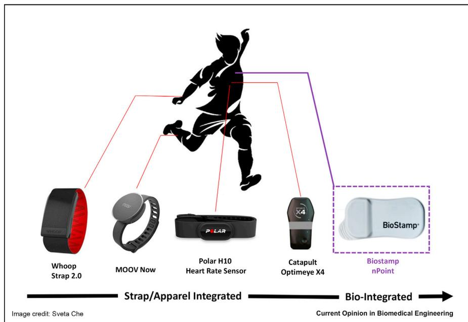
Representative commercial devices for athletic performance monitoring. Typical commercial embodiments exploit straps (Whoop Strap 2.0, MOOV Now, Polar H10) or integrate with apparel (Catapult Optimeye X4) to interface with the skin for monitoring athletic performance. The BioStamp nPoint (MC10 Inc.), harnessing recent advances in stretchable electronics, represents the first truly biointegrated commercially available platform for wireless athletic performance monitoring.
