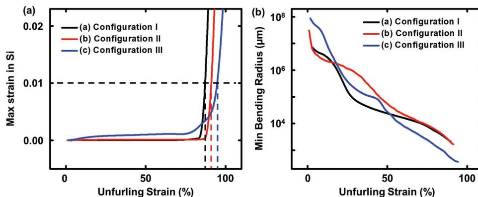
**Figure 3.** Mechanical simulations of flexible silicon transient optical waveguides. a) Plot of maximum strain in the Si as a function of unfurling strain for each configuration. A maximum strain of 1% corresponds to the fracture point of the Si. b) Plot of the minimum (out-of-plane) bending radius as a function of unfurling strain for each configuration.
