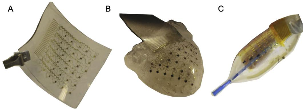
**Fig. 1. Custom Design Option.** Sample geometries for stretchable membrane devices. **A** planar sheet with gold recording electrodes. **B** Epicardial membrane custom design for rabbit heart geometry with gold recording electrodes. **C** Endocardial balloon with gold recording electrodes and IRO<sub>2</sub> pH electrodes.
