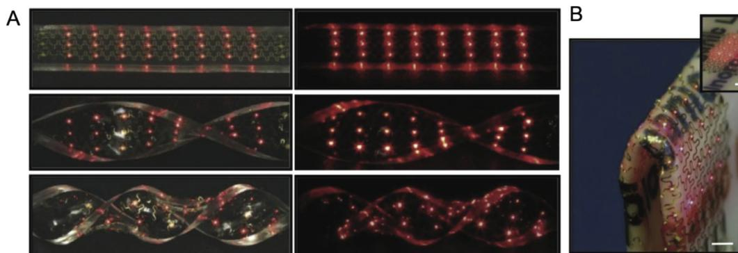
**Fig. 2. Conformability of circuits.** **A** LED circuit in the flat configuration and various degrees of twisting the substrate. Illumination demonstrates integrity of circuit is maintained. **B** LED circuit is bent around a corner. Illumination demonstrates integrity of circuit is maintained. This figure is modified from Kim et al., 2010.
