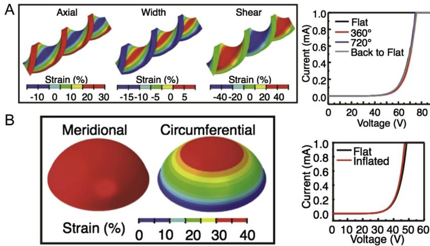
**Fig. 3. Representative Device Mechanics.** **A** Distributions of stain calculated by FEM for 720 degrees of twist and the I–V relationship during twisted and untwisted states. **B** Distribution of strain calculated by FEM for a configuration stretched by inflation and corresponding I–V relationship. Figure modified from Kim et al., 2010.
