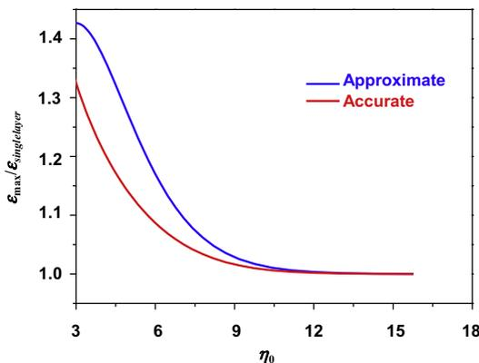
Fig. 3. Maximum strain  $\epsilon_{max}$  normalized by its counterpart  $2\sqrt{\epsilon_{pre}\epsilon_c/(1+\epsilon_{pre})}$  for a thick, single-layer substrate versus  $\eta_0$  for  $r = 1/20$ .
