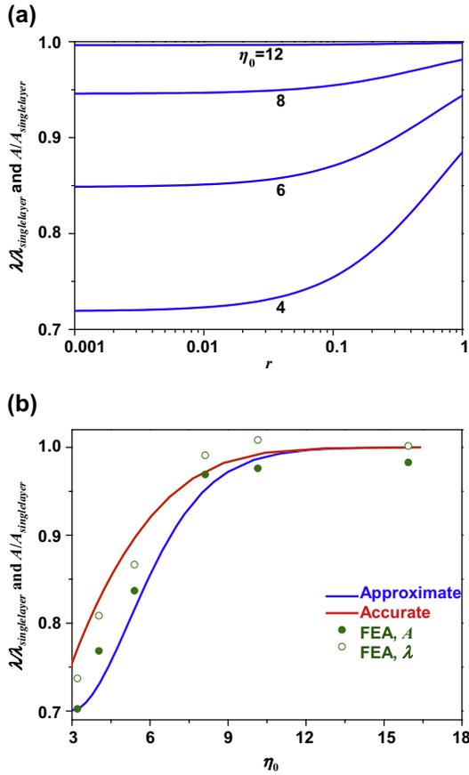
Fig. 2. Normalized wavelength  $\lambda/\lambda_{singlelayer}$  and amplitude  $A/A_{singlelayer}$  versus (a) the moduli ratio  $r$  of top to bottom substrate layers for different  $\eta_0$  values and (b)  $\eta_0$  for  $r = 1/20$ .
