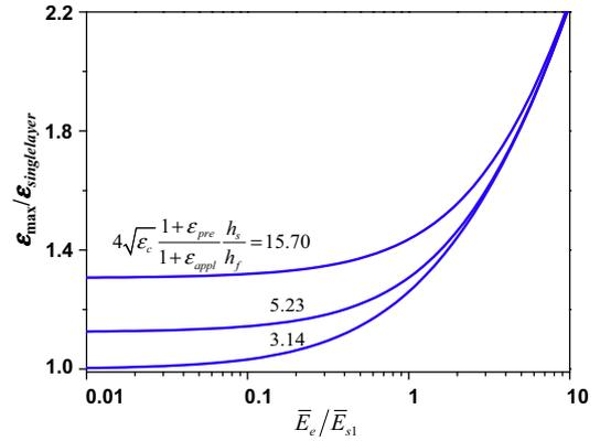
Fig. 5. In the case of encapsulation, the maximum strain  $\varepsilon_{max}$  normalized by its counterpart  $2\sqrt{(\varepsilon_{pre} - \varepsilon_{appl}) \bar{E}_c / (1 + \varepsilon_{pre})}$  for a thick, single-layer substrate without encapsulation versus the moduli ratio  $\bar{E}_e / \bar{E}_{s1}$  of the encapsulation to top substrate layers for different values of  $4h_s(1 + \varepsilon_{pre})\sqrt{\bar{E}_c} / [h_f(1 + \varepsilon_{appl})]$ .
