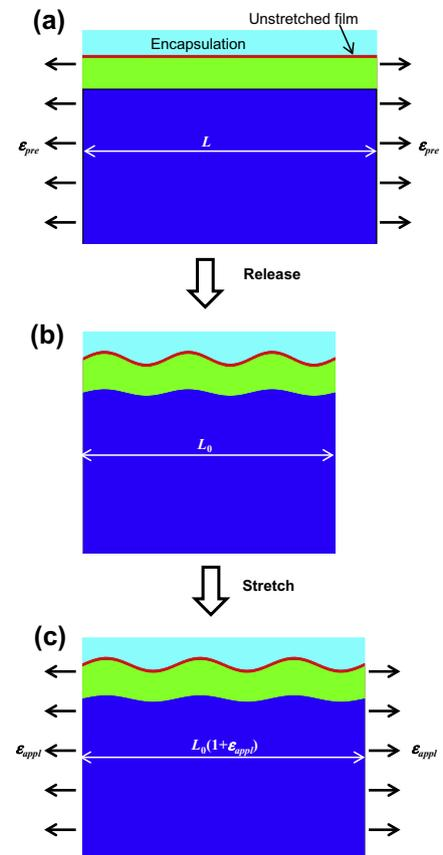
Fig. 4. Schematic illustration of the buckled system with encapsulation layer.
