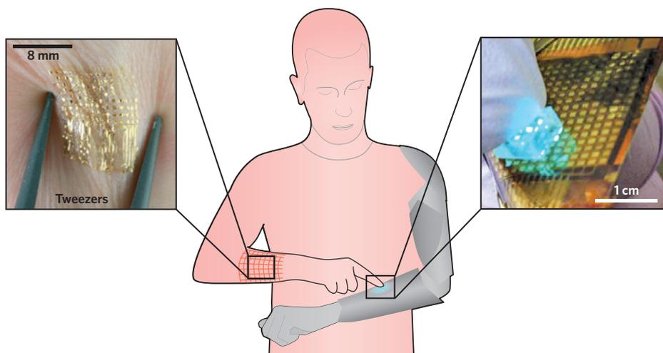
**Figure 1** | Humanoid robots in science fiction inspired the development of electronic skin with a sensory perception similar to that of humans. Left: Ultrathin conformal electronic films on elastomeric substrates gently adhere to human skin, and follow the pinching of the skin in a twisting motion. Such films enable precision thermometry of the skin<sup>2</sup>. Right: Local light emission from the touched array illustrates a user-interactive touch panel<sup>1</sup>.
