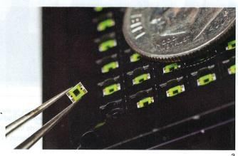
1/ Semprius's solar panels use glass lenses to concentrate incoming light, maximizing the power production of tiny photovoltaic cells.
