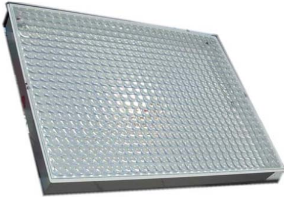
Power pack: Each Semprius solar panel is made of an array of 660 lenses that focus light on 660 tiny solar cells. Semprius
