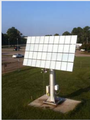
Solar tracker: This array of solar modules was built by Semprius for testing. The modules are mounted on a two-axis tracker that keeps them aimed at the sun. Semprius
