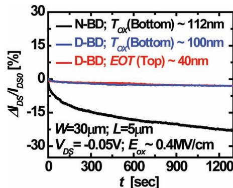
**Figure 7.** Percentage change in drain current ( $I_{DS}$ ) relative to the initial value ( $I_{DS0}$ ) as a function of time ( $t$ ), for three different CNTFETs. The bottom-gated CNTFET with significant levels of bulk defects near the nanotube (N-BD: black line) shows large degradation in  $I_{DS}$ . Devices with small bulk defects deep within the oxide (D-BD), both in bottom-gate (blue line) and top-gate configurations (red line), show comparatively small degradation in  $I_{DS}$ .
