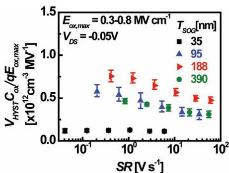
**Figure 3.** Plot of normalized  $V_{\text{HYST}}$  as a function of  $SR$  for top-gated CNTFETs (Figure 1c) with different SOG thicknesses ( $T_{\text{SOG}}$ ). Decreases in  $V_{\text{HYST}}$  with  $SR$  suggest the presence of bulk defects (more for thicker SOG) within the SOG/ $\text{HfO}_2$  dielectric.
