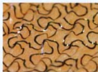
THE CIRCUITS' FILAMENTARY SERPENTINE SHAPE ALLOWS THEM TO BEND, TWIST, SCRUNCH AND STRETCH WHILE MAINTAINING FUNCTIONALITY
