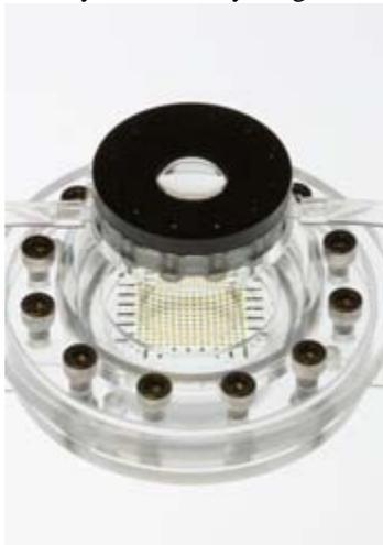
The "eyeball camera" has a 3.5x optical zoom, takes sharp images and is only the size of a nickel.
