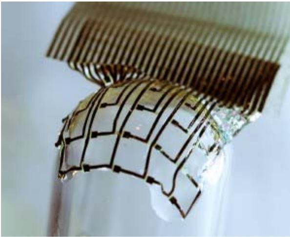
The research team printed electrode arrays onto silk films that disintegrate after they are placed on the brain's surface and flushed with saline. They're just 2.5 microns thick, so thin that they need to rest on a platform so they don't fall apart during fabrication or implantation. After the silk film dissolves, the array wraps around the curves on the brain.
