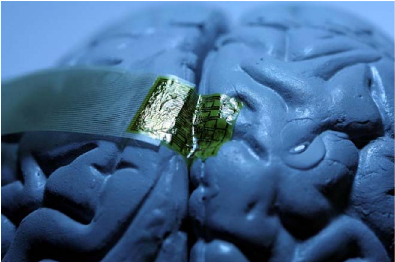
Silk has made its way from the soft curves of the body to the spongy folds of the brain. Engineers have now designed silk-based electronics that stick to the surface of the brain, similar to the way a silk dress clings to the hips.
