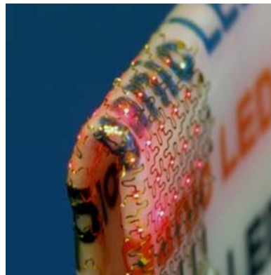
A LIGHT READ: A flexible array of LEDs on a folded sheet of paper. Image: COURTESY OF JOHN A. ROGERS
