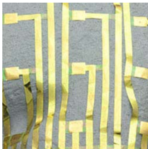
Neural electrode array wrapped onto a model of the brain. The wrapping process occurs spontaneously, driven by dissolution
