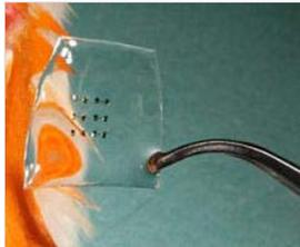
**Silk-Silicon Electronics** Silk substrates fitted with ultra-thin silicon transistors can be implanted to conform to the body's tissues, opening the door for enhanced implantable medical devices of various uses. The silk dissolves harmlessly overtime, leaving the silicon circuitry behind (the orange liquid in the photo is a disinfectant used during the implanting procedure). *Rogers/Omenetto*
