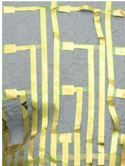
Neural electrode array wrapped onto a model of the brain. The wrapping process occurs spontaneously, driven by dissolution of a thin, supporting base of silk. (Image: C. Conway and J. Rogers, Beckman Institute)
