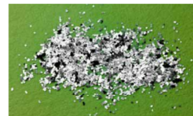
A pile of gallium arsenide solar cells manufactured in stacks and then peeled apart layer by layer. They can be integrated into a number of electronic devices. © John Rogers
