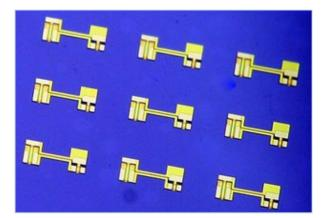
The small size of the thin silicon circuits avoids adverse biological reactions while the silk conforms to tissue and dissolves harmlessly over time, factors that make the technology ideal for safely integrating biomedical devices into the human body.
