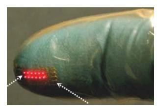
Position sensors on a surgical glove. The arrows point to the light-emitting (left) and photodetector part (right) of the position sensing array. Reprinted by permission from
