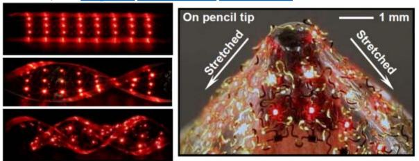
Stretchable electronic arrays. The LED sheets can be twisted by 720 degrees and considerably stretched. The wavy metal wires are visible in the image on the on the right. Reprinted by permission from Macmillan Publishers Ltd. Nature Materials (2010). doi:10.1038/nmat2879
