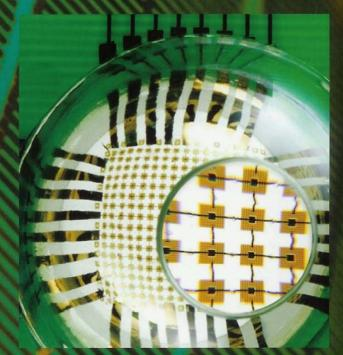
The same technology that creates "flexible" solar cells is being applied to other devices, such as a high-performance, hemispherical "eye" camera using an array of single-crystalline silicon detectors and electronics, configured in a stretchable, interconnected mesh.
