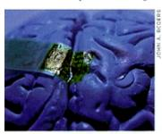
Y BUILDING ELECTRONICS on substrates of silk, scientists have created devices so thin and flexible that they hug the brain's ridges and grooves (Nat. Mater., DOI: 10.1038/nmat2745). The
