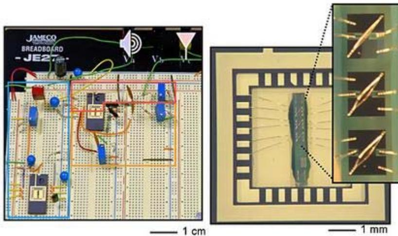
Image of the nanotube-transistor radio, which magnified views of carbon-nanotube transistors wire bonded into dual in-line packages.
