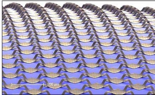
The curved detection surface, made of 'stretchable electronics', works like a human eye
