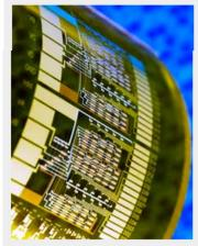
Fast and flexible: An integrated circuit on a thin plastic sheet incorporates transistors made from single-walled carbon-nanotube networks. The carbon-based networks rival the performance of single-crystal silicon, but they can be easily printed onto the plastic from solution and have good mechanical properties that are useful for flexible electronics. Credit: Beckman Institute, University of Illinois
